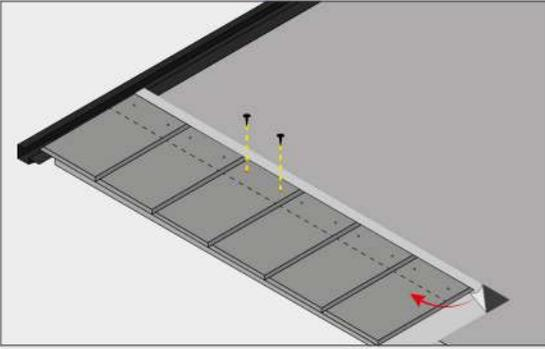
Lay the first READYSLATE® panel down and nail each piece of slate using the pre-punched holes provided. Once the panel install is complete, peel back the protective film on the top and right side of the panel.
