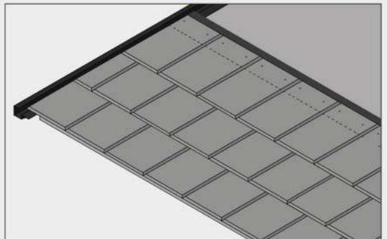
Readyslate's innovative design allows the panels to be installed on almost any roof type. Upon completion, you are left with a beautiful, durable, waterproof, and eco-friendly natural slate roof.
