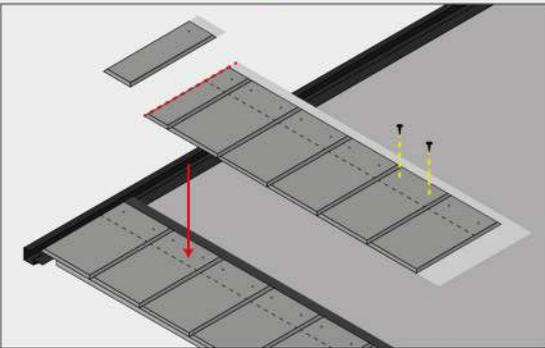
READYSLATE® is designed with an overlap line that allows for quick and easy placement of each panel.
